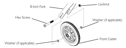
FIGURE 8.2 Replacing Front Casters
